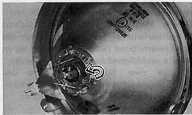
3. Unhook the headlight bulb spring retainer as shown and remove the defective bulb from the headlight lens unit.
