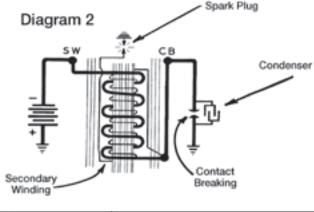
duction in the voltage required to break down the plug gap. If the car is converted to negative ground and if a negative ground coil is not installed, the 10 percent advantage is lost. This effect can be seen if you attach a scope to your car. The picture of the HT system would be upside down. If you change to a negative ground, it is always better to replace the coil with a negative system coil.
